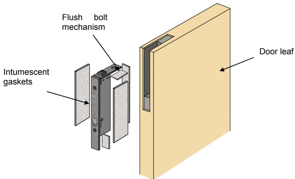
2. Bolts may be installed with no protection provided that the fitted meeting edge intumescent seals are either:
