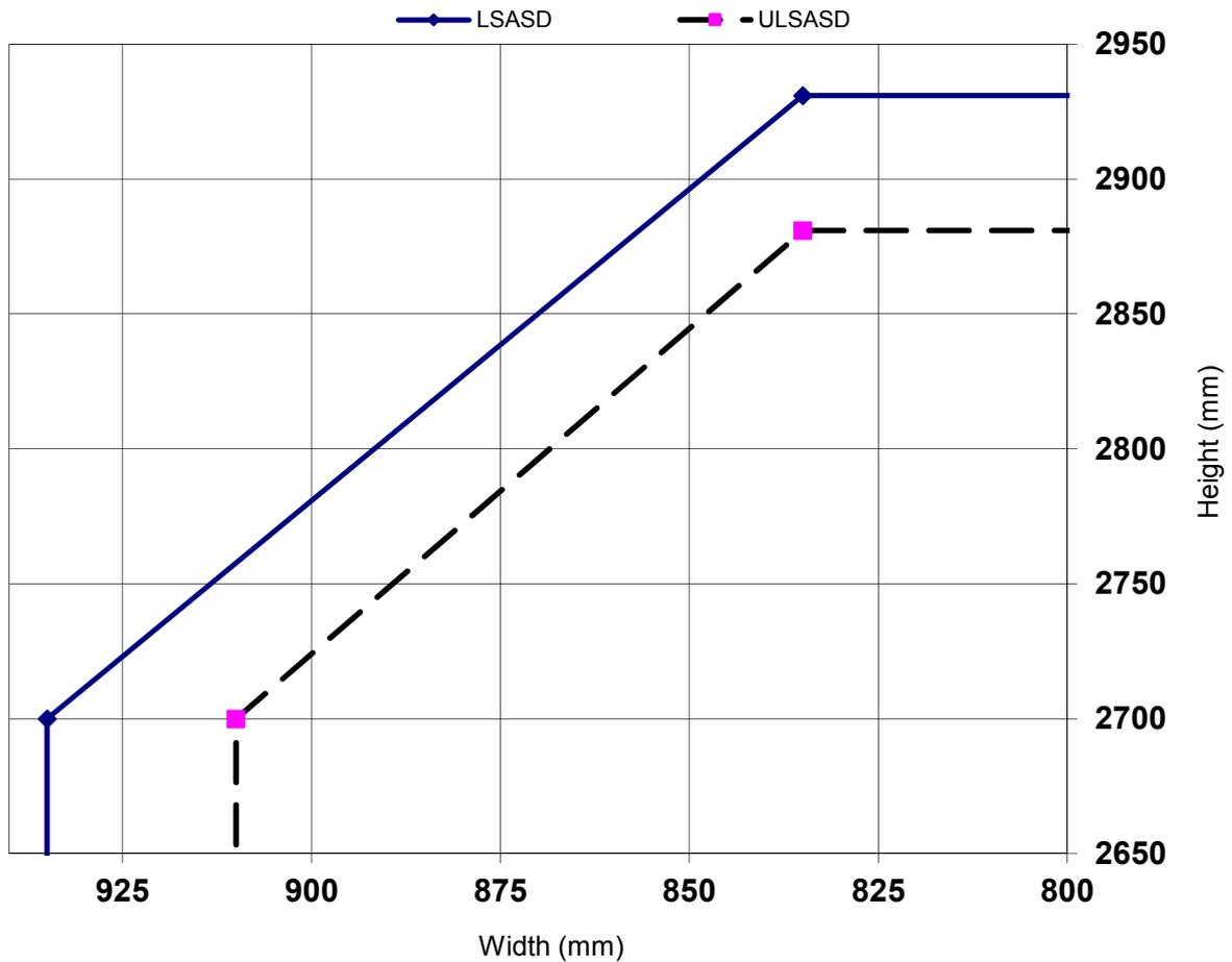
**Halspan® 30 Optima Doorsets - Aluminium Frame Doorsets – FD30 Rating**
