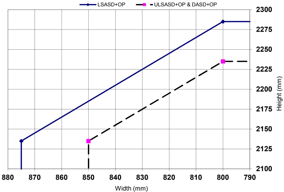
**Halspan® 30 Optima Doorsets - Backfilled Steel Frame Doorsets – FD30 Rating**
